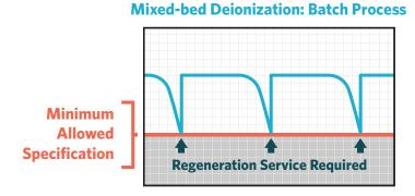
As ion-exchange resins exhaust, contaminants begin to break through, eventually requiring downtime for resin regeneration or replacement.
