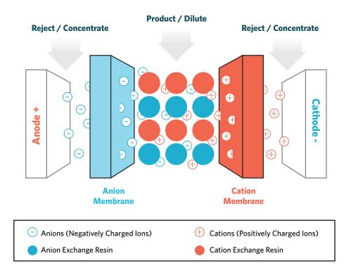
CEDI is a chemical-free, self-regenerating technology used to provide a consistent flow of high-quality deionized water.
