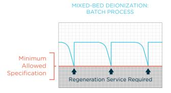
As ion-exchange resins exhaust, contaminants begin to break through, eventually requiring downtime for resin regeneration or replacement.
