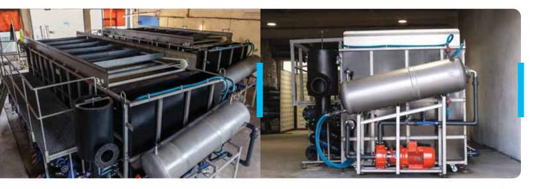
Fully assembled Dissolved Air Flotation (DAF) system designed for a flow capacity of 60 m³/h. Equipped with air injection, flotation, and sludge removal systems for efficient wastewater treatment. Pre-tested and ready for installation at the client's site.
