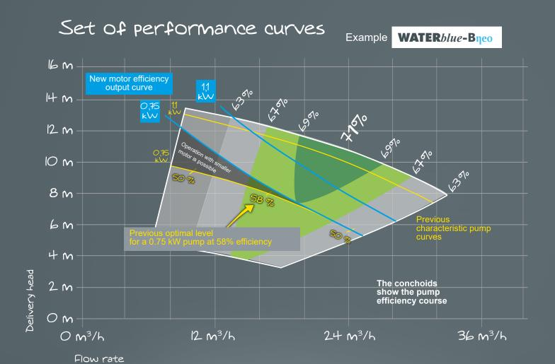
Example for 0.75 kW pump: Previous optimal efficiency level: 58 % New efficiency with full impeller diameter according to shell curve: 68 % => Hydraulic optimisation of the efficiency by 10 %!
