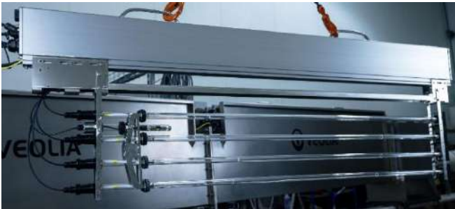
Figure 2: Four lamp module with power bar
